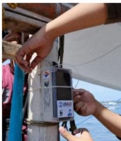
Installation of FAME transponder to a small-scale tuna handline fishing vessel. Photo: David N. David / WWF-Philippines
